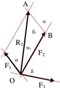
$$F_1 = 2000 \text{ N}, F_2 = 3000 \text{ N}, F_3 = 2500 \text{ N}, \alpha = 68^\circ, \beta = 75^\circ$$
