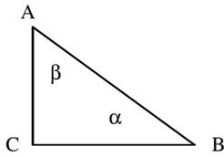
$$\overline{AB} = \sqrt{\overline{AC}^2 + \overline{BC}^2} = \sqrt{30^2 + 50^2} = 58,3 \text{ mm}$$
