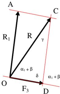
$$R = \sqrt{R_1^2 + F_3^2 + 2R_1F_3 \cos(\alpha_1 + \beta)} = \sqrt{4182,73^2 + 2500^2 + 2 \times 4182,73 \times 2500 \cos 101,31^\circ} = 4431,83\text{N}$$
