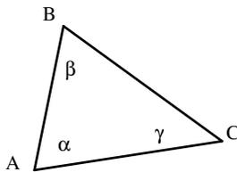
$$AC = \sqrt{AB^2 + BC^2 - 2 \cdot AB \cdot BC \cdot \cos \beta} = \sqrt{40^2 + 60^2 - 2 \times 40 \times 60 \times \cos 65^\circ} = 56,31 \text{ mm}$$
