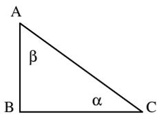
$$\overline{BC} = \sqrt{\overline{AC}^2 - \overline{AB}^2} = \sqrt{110^2 - 60^2} = 92,19 \text{ mm}$$
